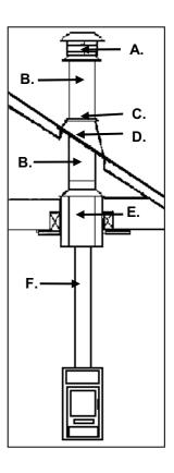
For venting vertically into a Class A chimney, single wall pipe (at least 24 gauge) may be used in the room where the stove is installed. Refer to the manufacturer's instructions for the connection to the listed chimney. The chimney/stove pipe must not be smaller than 6" (15cm) in diameter.
